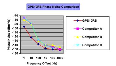
The graph to the left shows the GPS10R/RB phase noise (red trace) compared with three competitors (Pink, Yellow, Blue traces). As can be seen the GPS10R/RB has lower phase noise than its competitors.
